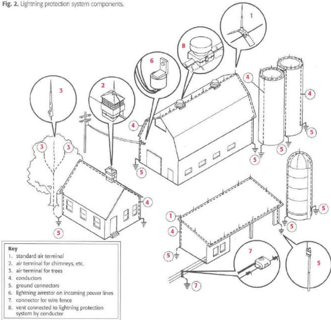
The best method for eliminating lightning-induced sideflashes between metal bodies is common grounding. This means that the grounds for all the electrical systems, the telephone service, and underground metal piping are connected to the lightning protection system. Plastic piping, which has become common in recent years, does not conduct lightning's electrical charges and requires special grounding.
