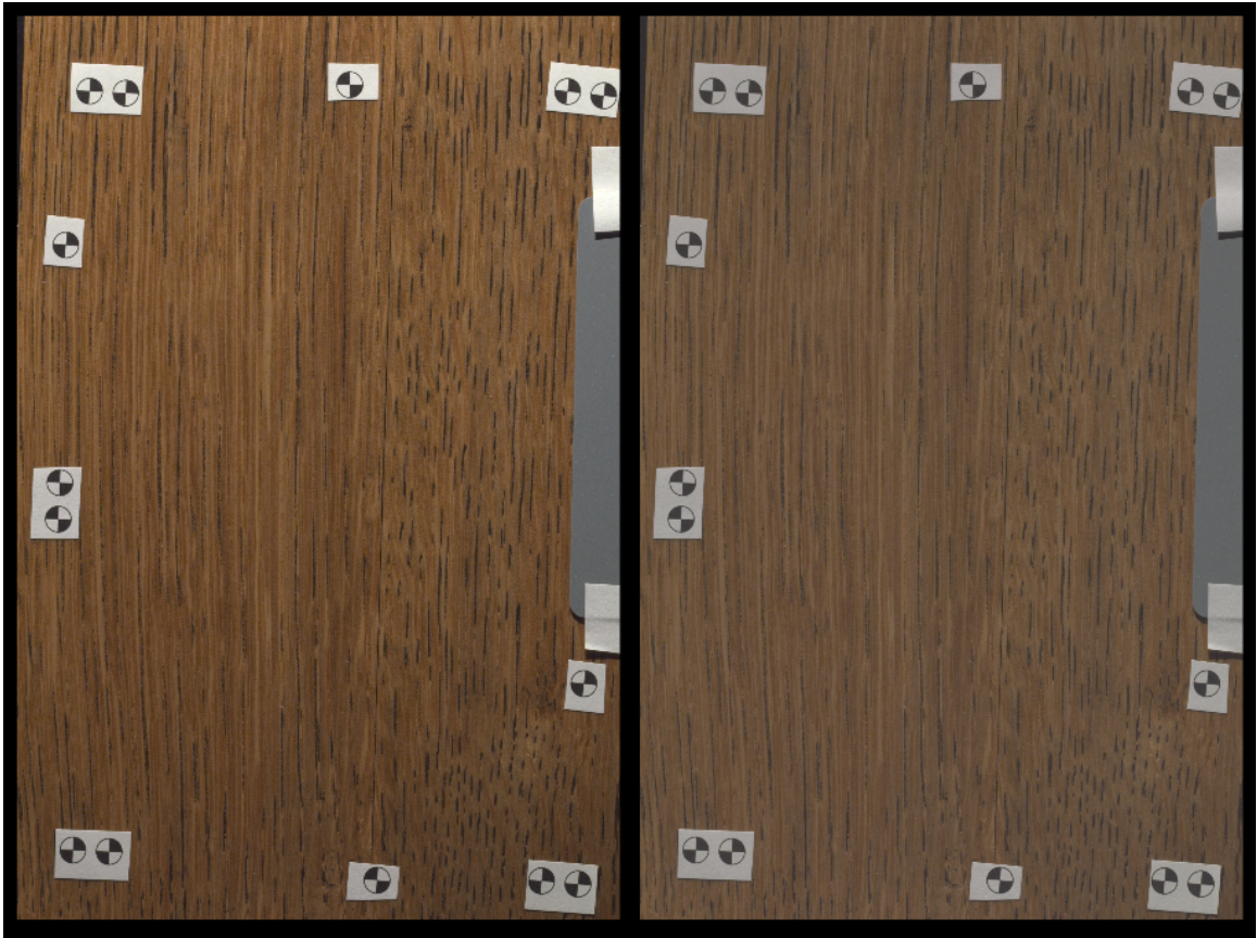
Figure 3.15: Irradiance Correction: the captured data is scaled using the incident illumination to recover measured BRDF values
