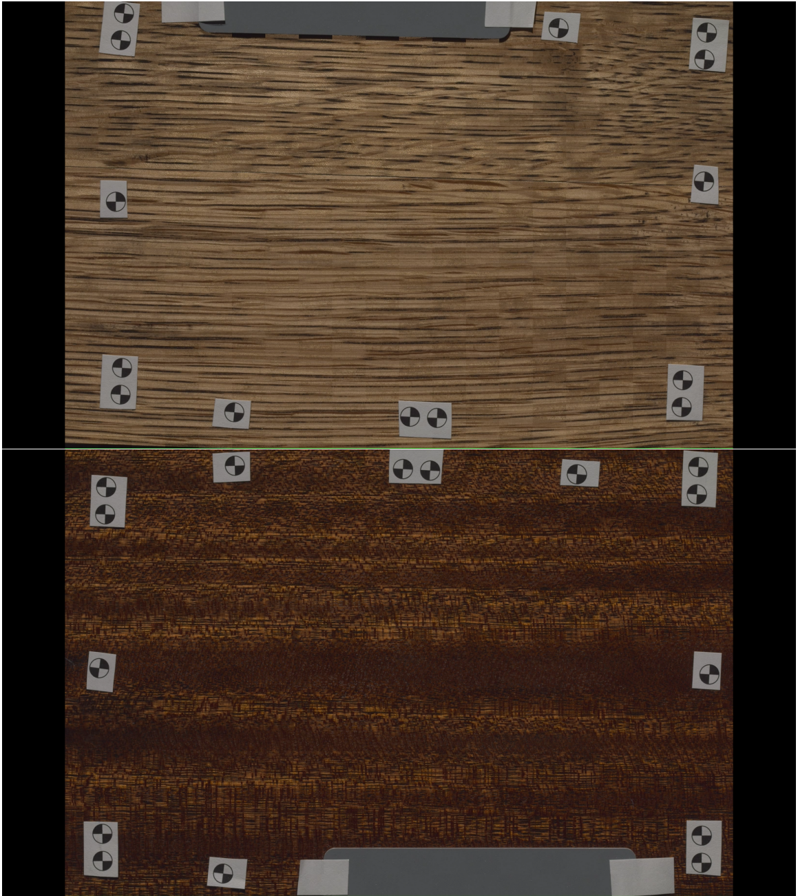
Figure 4.2: Checkerboard Comparison of Fitted Result to Measurement Data (top image oak; bottom image mahogany). Note the grid boundaries are barely visible indicating a close match
