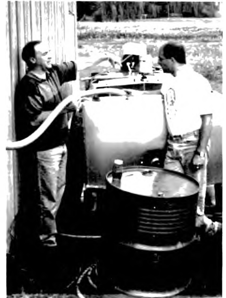
Bob Kime talks to Chris Stamp about the mixture of honey and water in the mixing tank before it is pumped into the holding tank for ultrafiltering.
