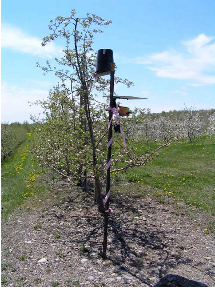
Figure 2. Weather station used to collect temperature and rainfall data in Newark, NY. Orchard is planted to Gala apple trees.
