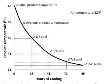
Figure 2.1. A cooling curve for a perishable product in room cooling.
