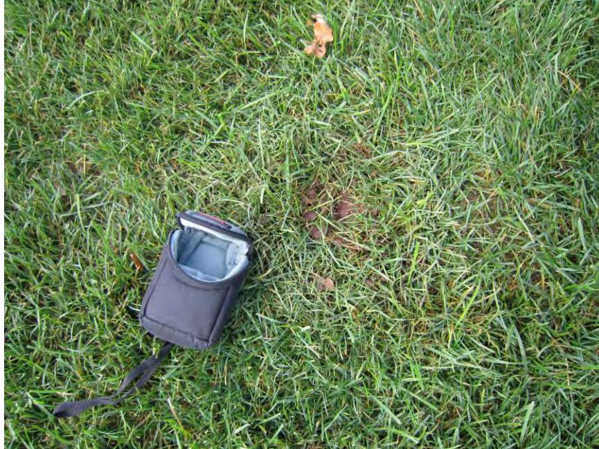
Figure 6 Surface disruption to golf course rough following Air injection treatment
