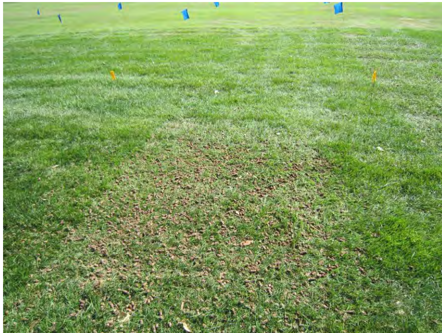
Figure 7 Surface disruption to golf course rough following 2 passes with ProCore (1/2" diameter hollow tines, 1.5" forward spacing)
