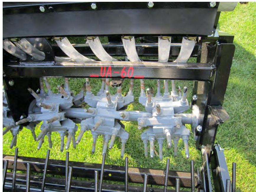
Figure 2 Tractor mounted solid, vibratory-tine cultivator (First Product UA-60)
