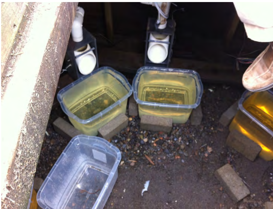
Photo 2: Chamber holding the lysimeter devices that collect drainage waters from the turf plots
