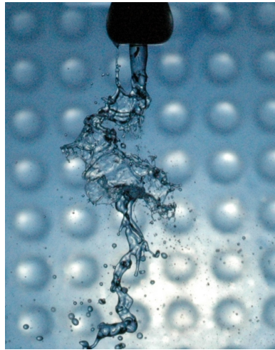
Figure 6.16: Example of nozzle wetting and the effect on break-up process.
