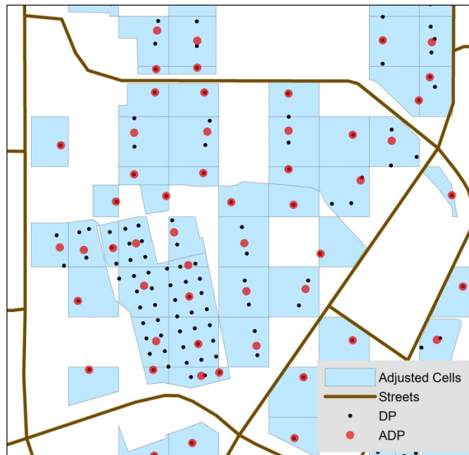
Figure 3-18 Aggregation results: locations of 37 approximating demand points and 90 demand points in the sampling block
