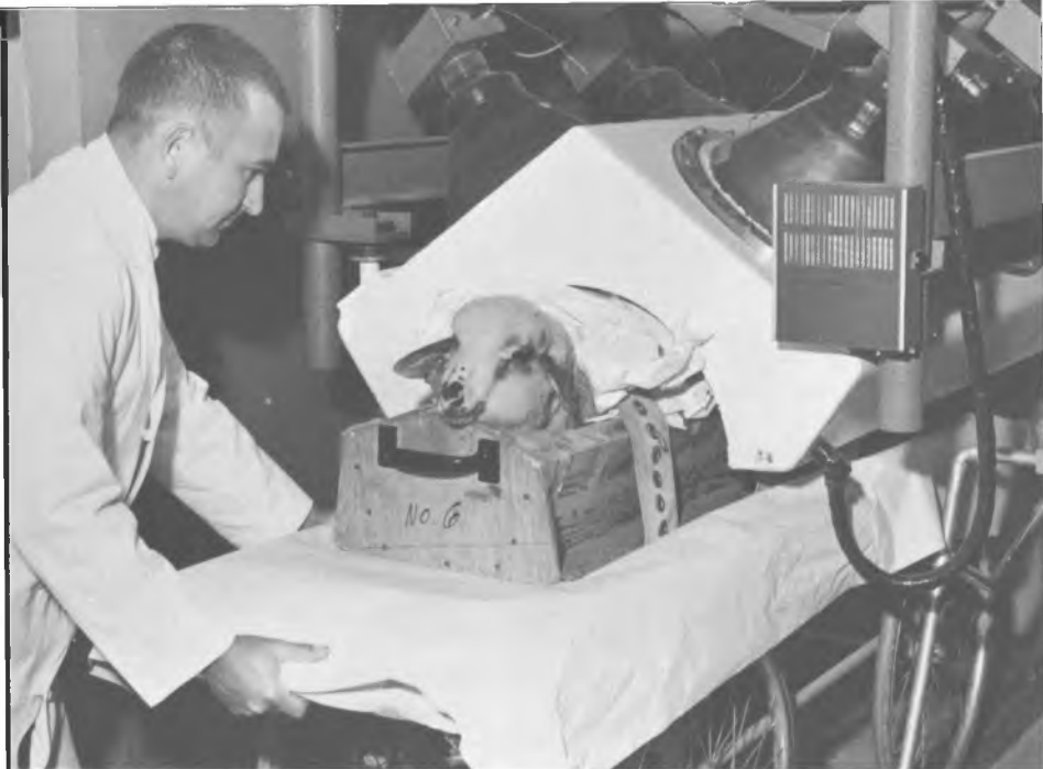
Positioning a lamb in the total body counter (Laboratory of Radiation Biology, Department of Physical Biology).
