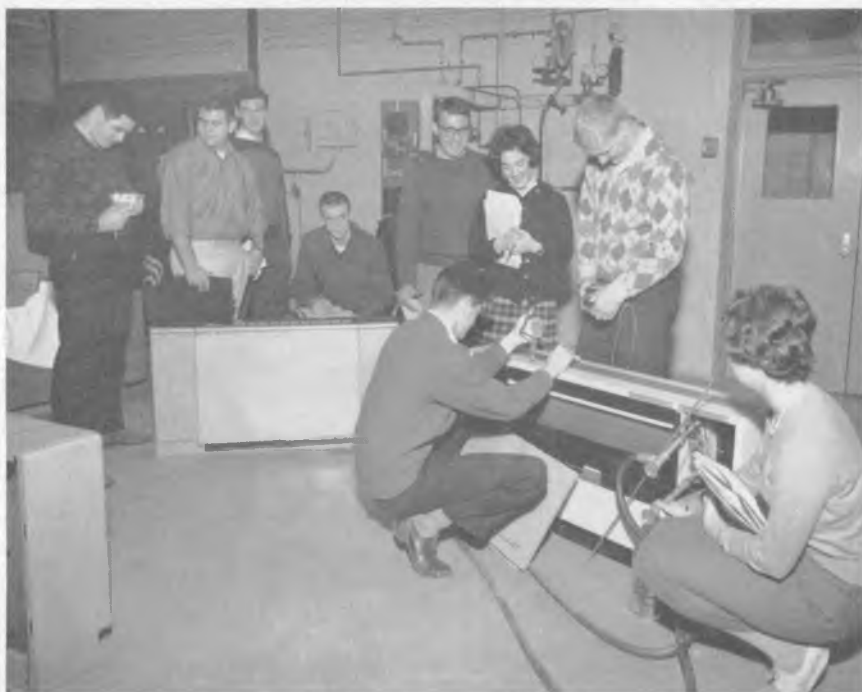
Achieving a comfortable environment for the guest is one of the primary objectives in selling guest space. Hotel administration students regularly participate in laboratory work involving heating, refrigeration, and air conditioning. Performance of various guest room fan coil units is being verified in the exercise shown above.
