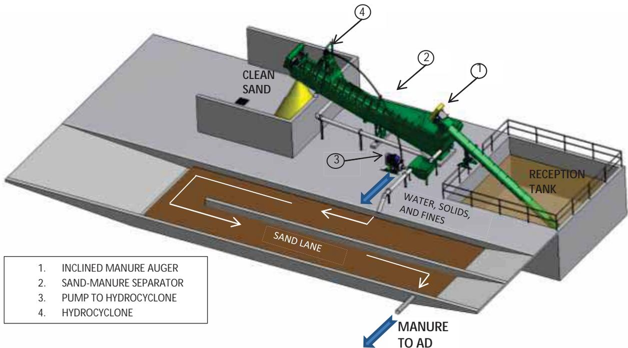
Figure 4: Sand-manure separation (SMS) system process flow.
