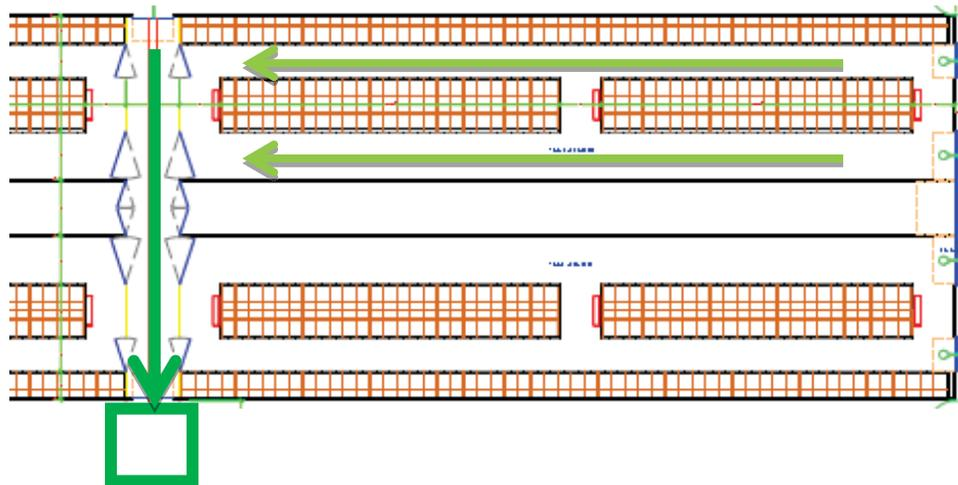
A flush flume system utilizes fast flowing liquid to transfer manure across the width of a barn or across several barns in a round tube. A high volume pumps creates an adequate flow rate to prevent settling of manure solids and bedding material. Water addition, and separation or dewatering is needed before evacuating to further processing to have enough liquid to keep the flush flume operating. Solids content of a flush flume will typically vary between 4 to 9% total solids.
