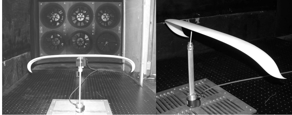
Figure 10: Quasi-static wind tunnel model and setup
