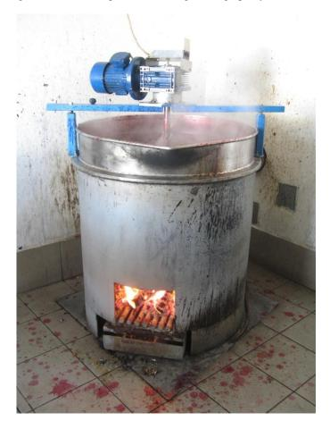
Figure 10. Motorized stirring pot. Photograph by Olivia Hall
