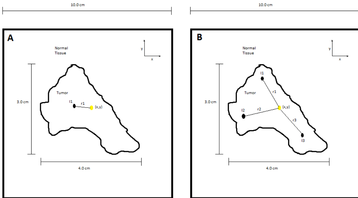
Figure 2: Schematic showing tumor geometry and location of (a) single injection site and (b) multiple injection sites. At a point (x, y) the volumetric heating term, Q , is a sum of the exponential distributions from each injection site I_1, I_2, I_3 .
