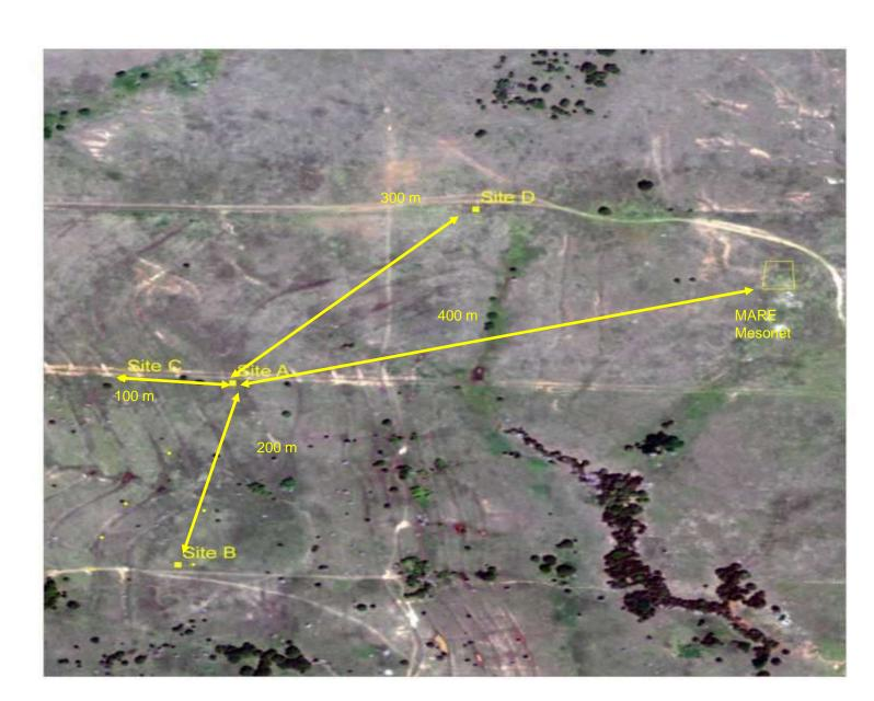
The testbed was organized around Base Sites which would hold a variety of sensors at different depths. There are 4 Base Sites, and additional instrumenation was added to these facilities.
