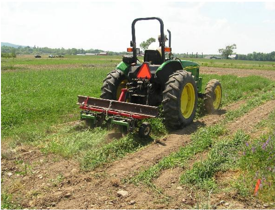
Figure 3.2: System 4 (Ridge-till) scraping ridges with hairy vetch before planting cabbage
