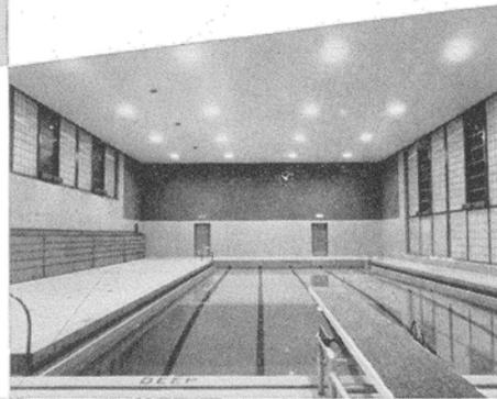
Kirlin #1212 R-W 300 W fixtures were used in the Allen Park (Michigan) High School pool. The architects, Eberly M. Smith Associates, secured 14 f.c. intensity uniformly on the water due to the wide angle lens even though fixtures border edge of pool for relamping from below.
