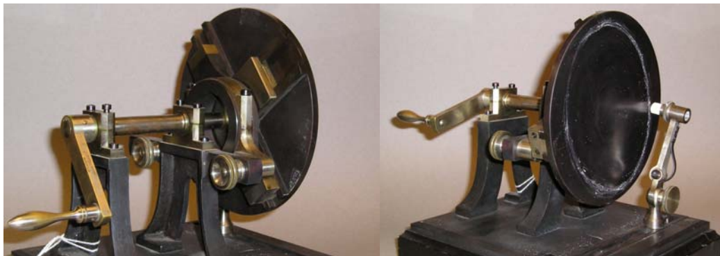
Figure 8. Trammel from Reuleaux kinematic model collection (photo Prof. D. W. Henderson)
