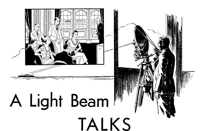
FROM the flickering light of a neon tube on the skyline of New York City, a speech was sent to the S. S. President Hoover, 3000 feet away. The small neon tube changed the electric impulses from a microphone into light waves, which were directed to the ship in a narrow beam. A photoelectric tube in the center of a receiving mirror on the ship changed the light impulses back into sound, and the speech was heard on board.
