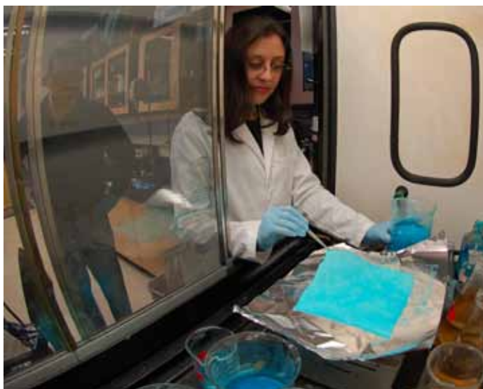
Postdoctoral associate Marcia Da Silva Pinto led the work to coat fabrics with metal organic molecules (MOFs).
