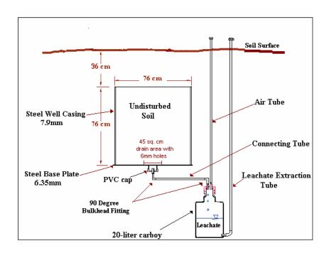
Figure 3: Lysimeter used to collect percolated water in each system in the Rodale Institute Farming Systems Trial.
