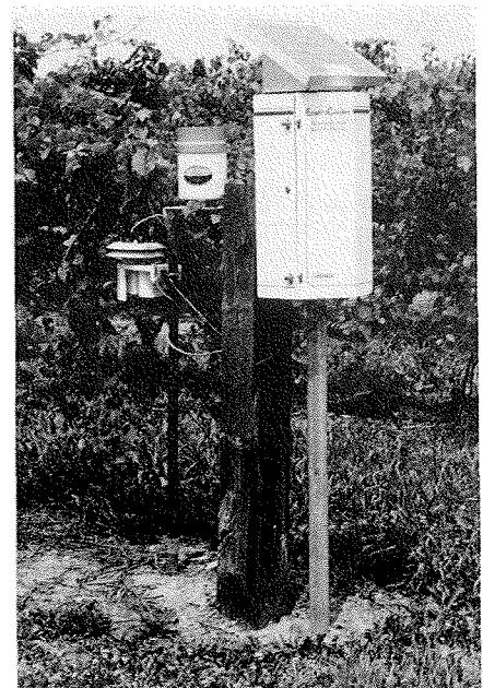
(B) A microprocessor-based instrument, which performs all of the functions of the modified hygrothermograph, and which contains programs for several disease forecasting models which use data collected by the instrument. A solar panel with battery backup provides power for the computer and printer contained within the weatherproof housing.
