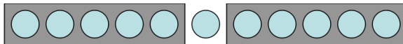
Figure 4.1: One-site DMRG block configuration. L^n tensors are associated with the left block, R^n tensors with the right block, and the middle site is site p in Eq. 4.1.
