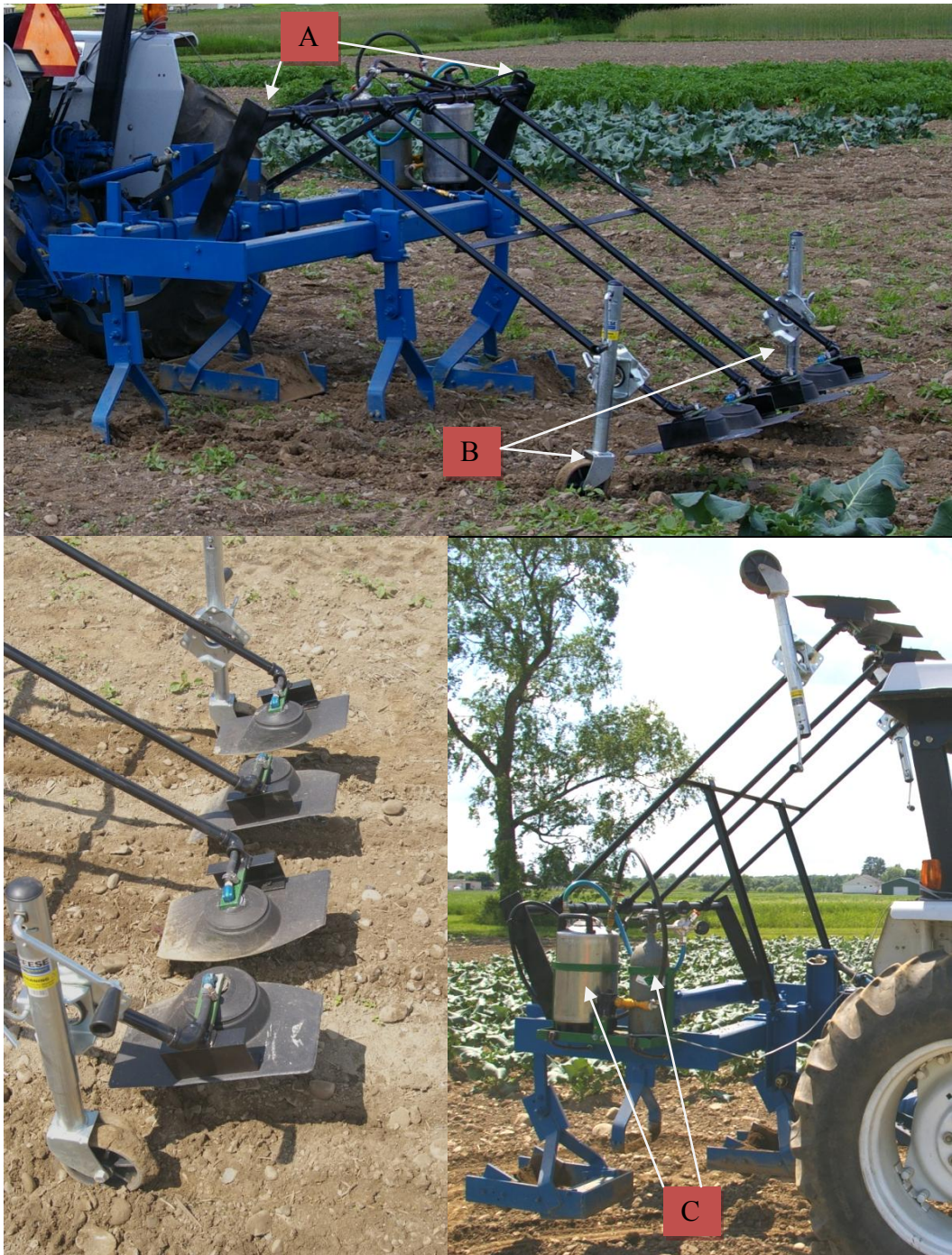
Figure 3.1. Images of the banded directed sprayer. Clockwise from the top: side view of sprayer (black) mounted to the rear of an inter-row cultivator (blue) with pivot points (A) and height-adjustable wheels (B); side view of sprayer raised in transport position with CO 2 pressure tank and vinegar holding tank (C); close-up of spray shield shape and orientation.
