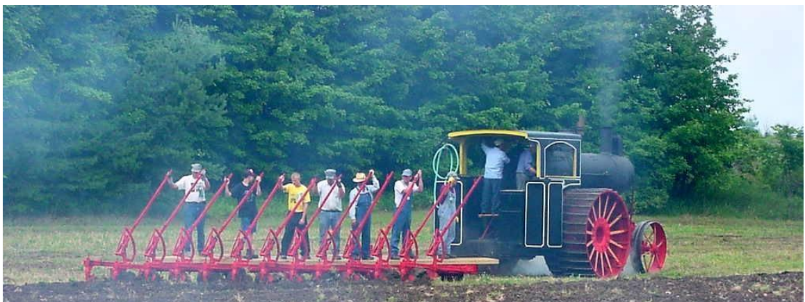
Figure 1.3. A restored steam tractor pulling a 12-gang plow. Note that this setup required operators on the plow to raise and lower each plow share as needed.
