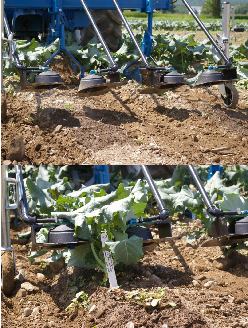
Figure 3.2. Images of the banded directed sprayer in action. Top: vinegar application in two 25-cm wide bands, with areas in-between cultivated; bottom: close-up of shields lifting broccoli leaves up and over the spray nozzles, while exposing weeds around the plant base.
