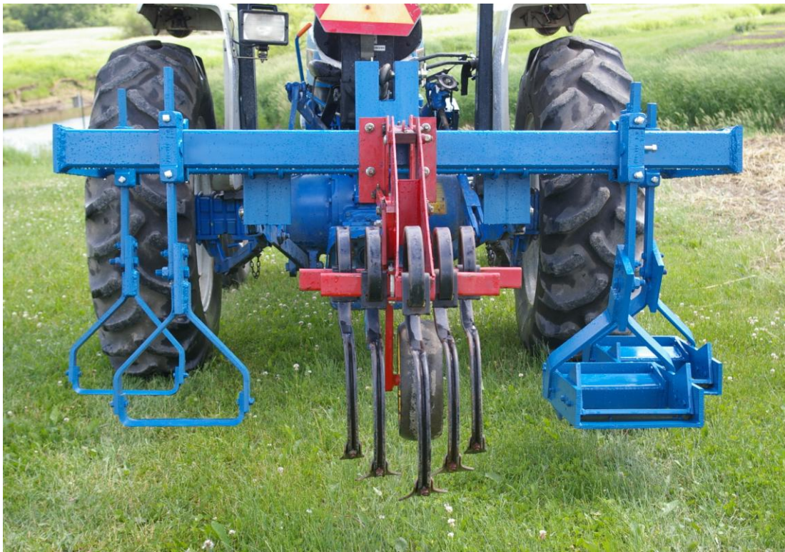
Figure 2.3. Rear view of the toolbar and the three different cultivator designs; from left to right: stirrup, sweep, and block cultivators.
