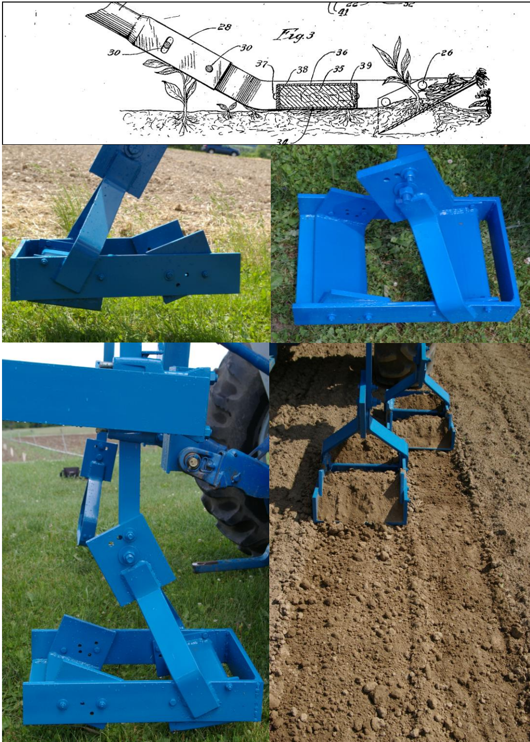
Figure 2.1. The block cultivator. Clockwise from top: original illustration of a hand tool designed in 1928 by M. Oakland; top-down view, with the front of the cultivator to the right; rear view, soil disturbance after cultivation; side view, showing the tool shank extending upward into a toolbar clamp and the toolbar attached to a tractor via a three-point hitch; side view of block cultivator, with the front of tool to the left.
