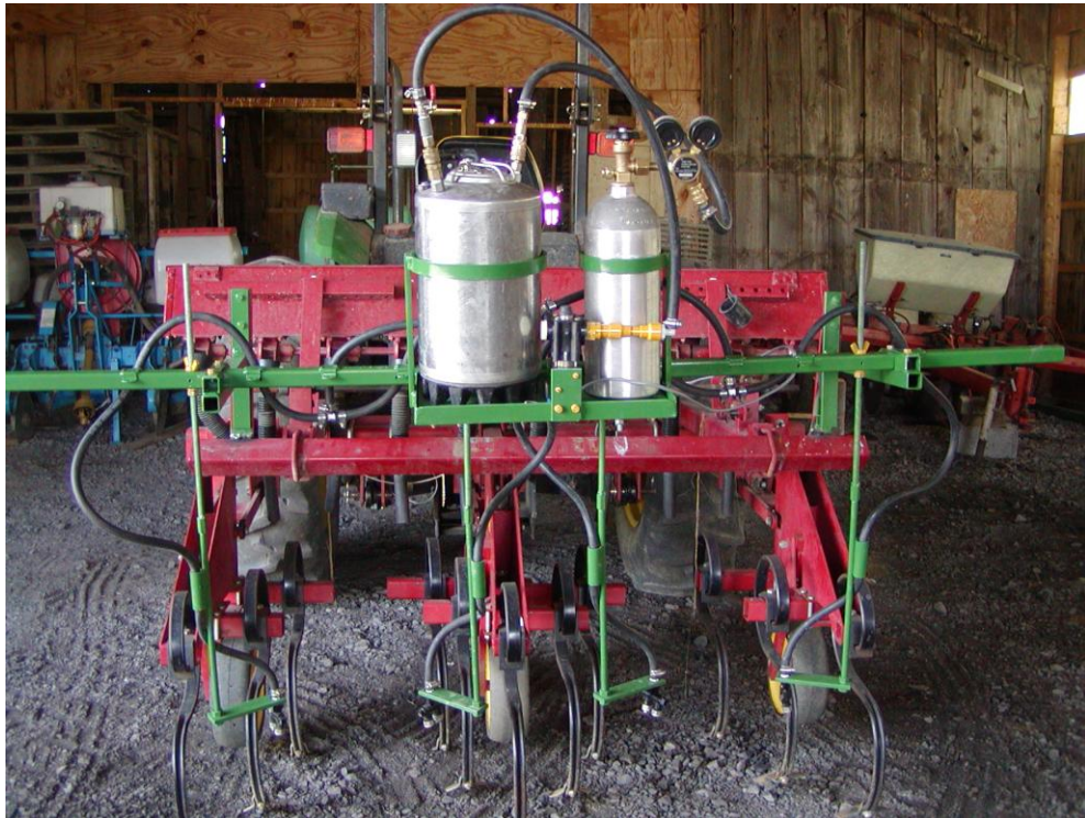
Figure A.1. Rear view of the sprayer. Sprayer structure is in green; the existing cultivator is in red.
