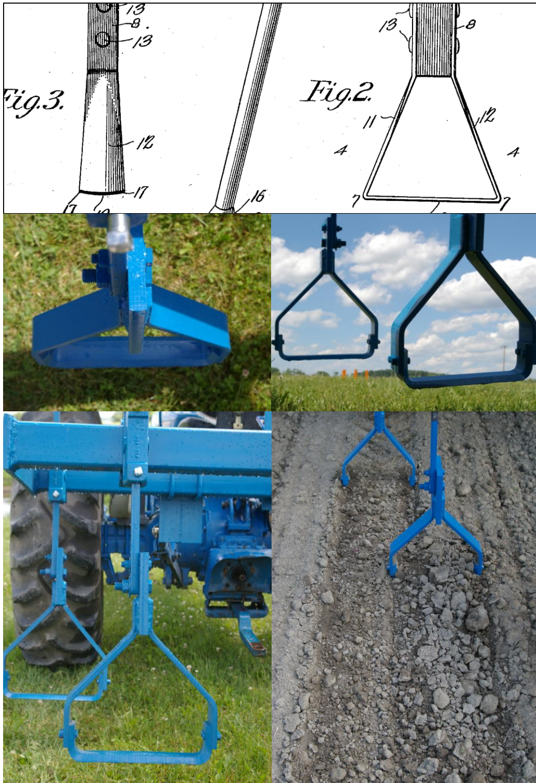
Figure 2.2. The stirrup cultivator. Clockwise from top: original illustration of a hand tool designed in 1903 by E. B. Morgan; front and side view; soil disturbance after cultivation; rear view of the cultivator, where the tool shank extends upward into a toolbar clamp; top-down view.
