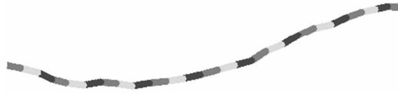
Figure 4.2: Modeled segment of LAD (20% of full length is shown): cylinders of different shades represent best matching templates stitched together
