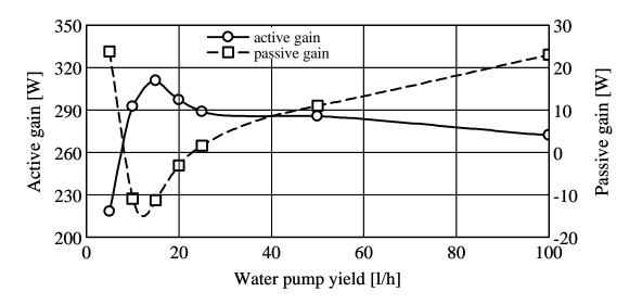
Figure 5. Relation between water pump yield and amounts of active and passive gain.
