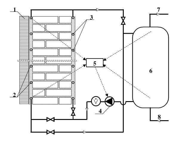
Figure 1. Hybrid wall scheme: 1- transparent thermal insulation, 2 - outer piping, 3- inner piping, 4- water pump, 5 - pump controller, 6 - water tank, 7 - hot water outlet, 8 - cool water inlet.
