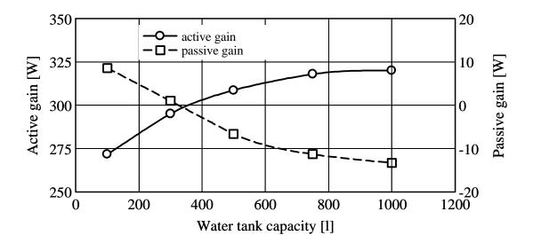
Figure 4. Relation of passive and active gain to water tank capacity.
