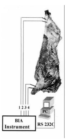
Figure 2. Diagrammatic presentation of BIA - system and optimum placement of drive (1.,4.) and measurement (3.,4.) electrodes.
