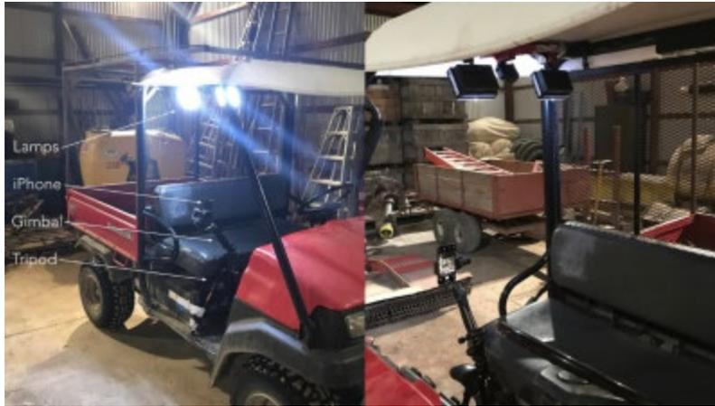
*A farm utility vehicle or atv can be modified for use in automatic sensing in vineyards by mounting a light panel and a smartphone on a gimbal. Photo by Jonathan Jaramillo.*
