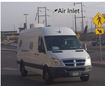
Figure 2 Air Quality Mobile Station
