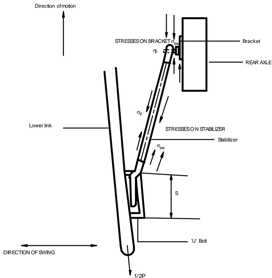
Figure 1. Steyr Tractor Three – point Hitch: Direction of movements of parts
