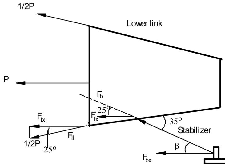
Figure 3. Forces Acting on the Lower Links and the Stabilizer
