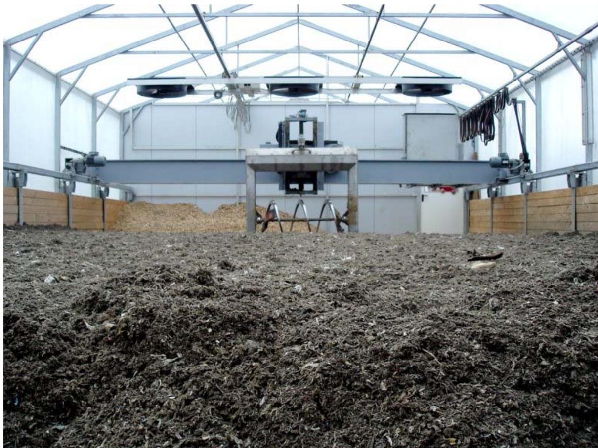
Figure 5. Prototype of the “Biomass-Manager” during an experiment in a solar greenhouse type dryer. The robot is processing a biowaste-paper blend.
