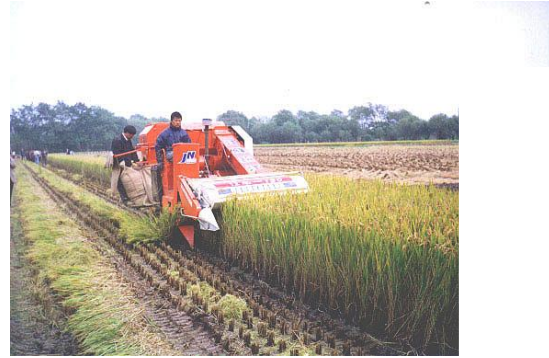
Figure 7 Stripping combine prototype in the experiment of harvesting rice
