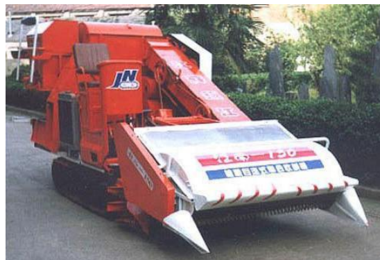
Figure 2 A trial prototype of 1.5 m wide stripping combine harvester with rubber-track driving device
