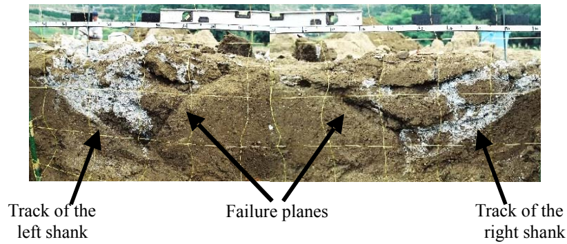
Figure 12. Cracking in the cross section of the field.
