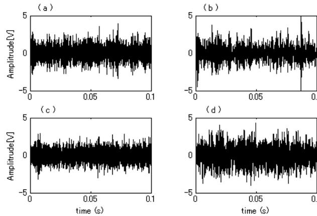
Figure 4. Original signals measured in each state: (a) Normal state, (b) Cavitation state, (c) Impeller damage state, (d) Misalignment state
