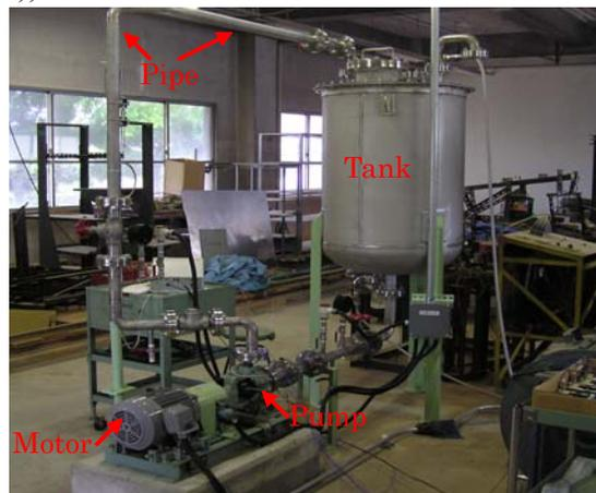
Figure 2. The experiment system of centrifugal pump in the field
