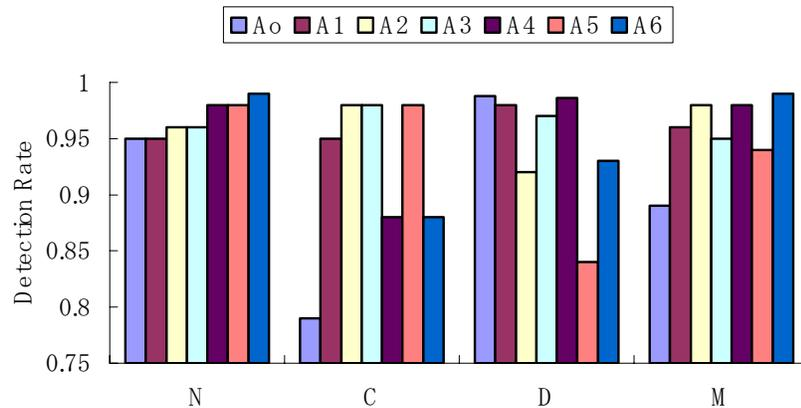
Figure 10. Detection rates in each state. N: Normal state, C: Cavitation state, D: Impeller damage state, M: Misalignment state.
