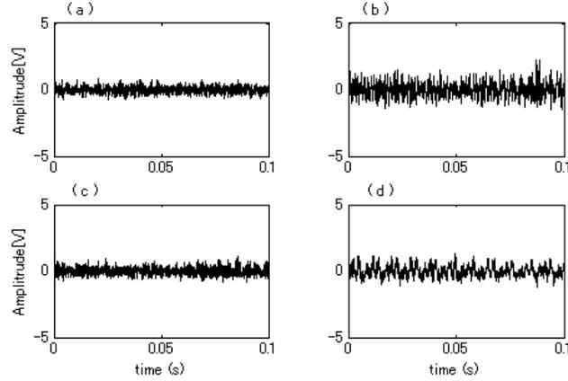
Figure 6. Recomposed signals in level 2 of each state: (a) Normal state, (b) Cavitation state, (c) Impeller damage state, (d) Misalignment state
