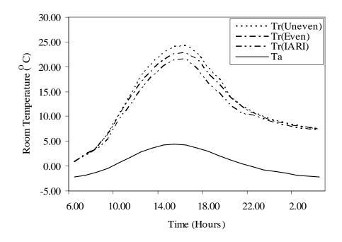
Figure 5 (b). Hourly variation of room air temperature in different shapes of greenhouse (with collector) at Srinagar.
