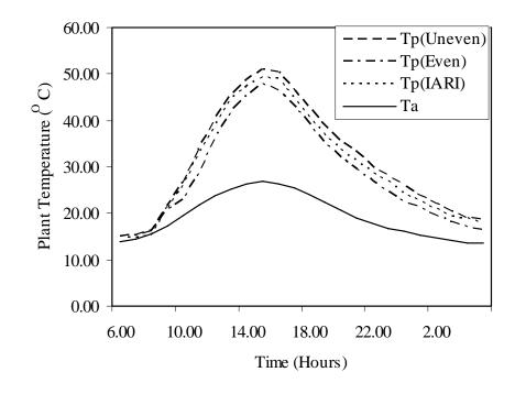
Figure 6 (a). Hourly variation of plant temperature in different shapes of greenhouse (with collector) at Kolkata.
