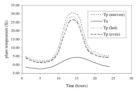
Figure 4 (a). Hourly variation of plant temperature in different shapes of greenhouse (with PCM North wall) at Srinagar.
