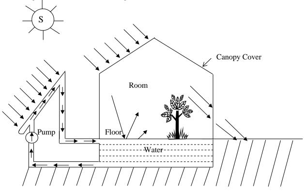
Figure 3(b). Schematic view of greenhouse with flat plate collector.
