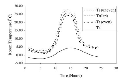
Figure 4 (b). Hourly variation of room air temperature in different shapes of greenhouse (with PCM North wall) at Srinagar.
