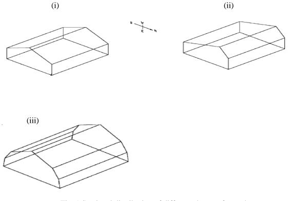
Fig. 1 Sectional distribution of different shapes of greenhouse (i) Evenspan (ii) Uneven span (iii) Modified IARI
