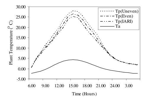
Figure 5 (a). Hourly variation of plant temperature in different shapes of greenhouse (with collector) at Srinagar.
