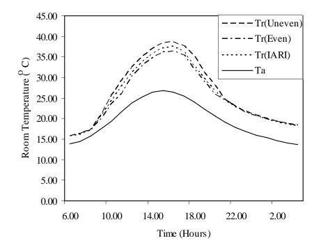
Figure 6 (b). Hourly variation of room air temperature in different shapes of greenhouse (with collector) at Kolkata.
