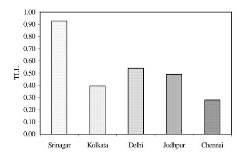
Figure 8. Variation of thermal load leveling (TLL) in even span greenhouse for different cities.
