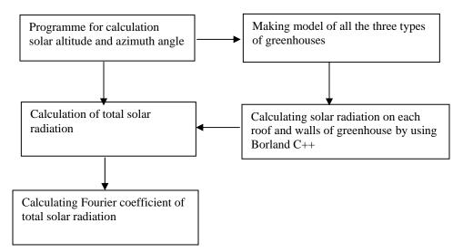
Fig. 2 Flow chart to calculate the total solar radiation.
