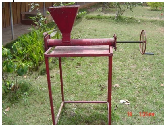
Figure 1: The manually operated briquetting machine
