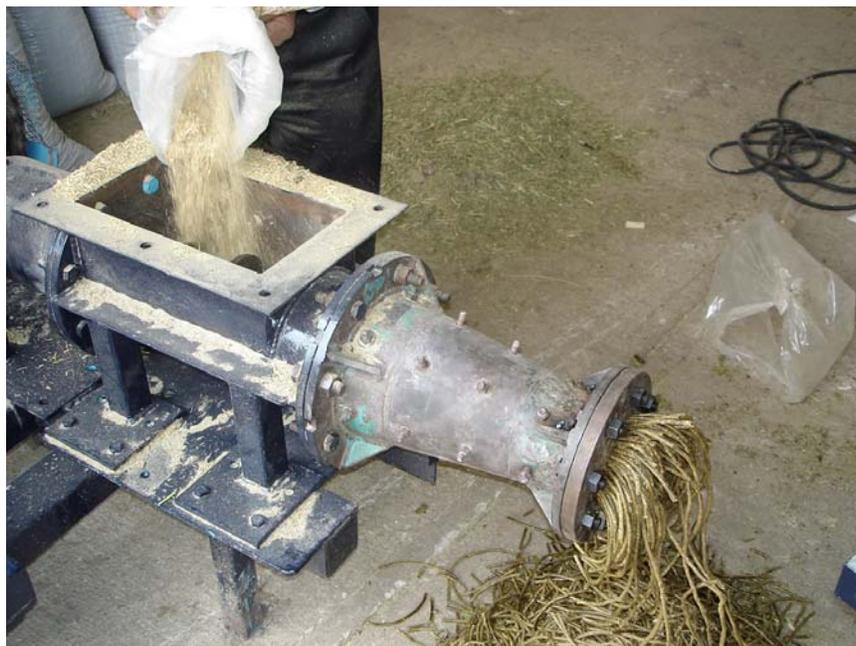
Figure 5. An extruder connected with rear power take-off of a tractor
