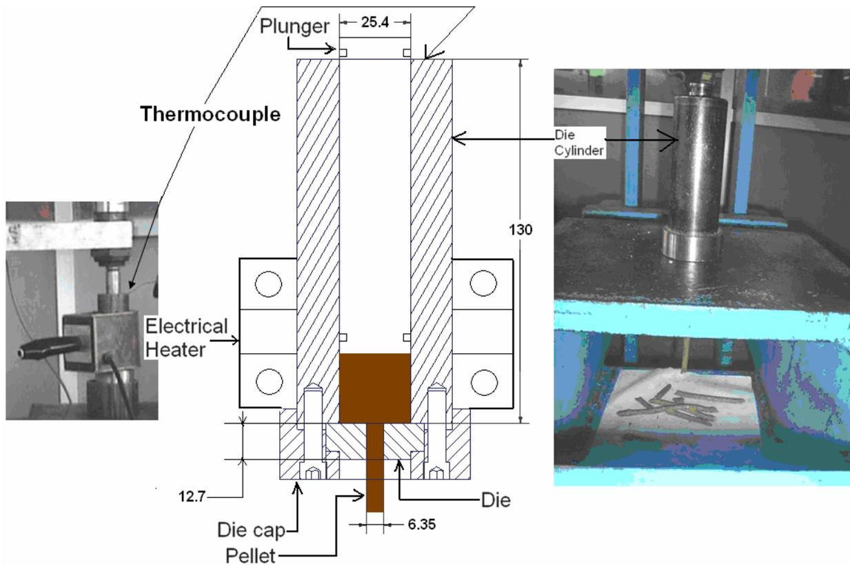
Figure 2. Densification open-end die (all dimensions in mm)
