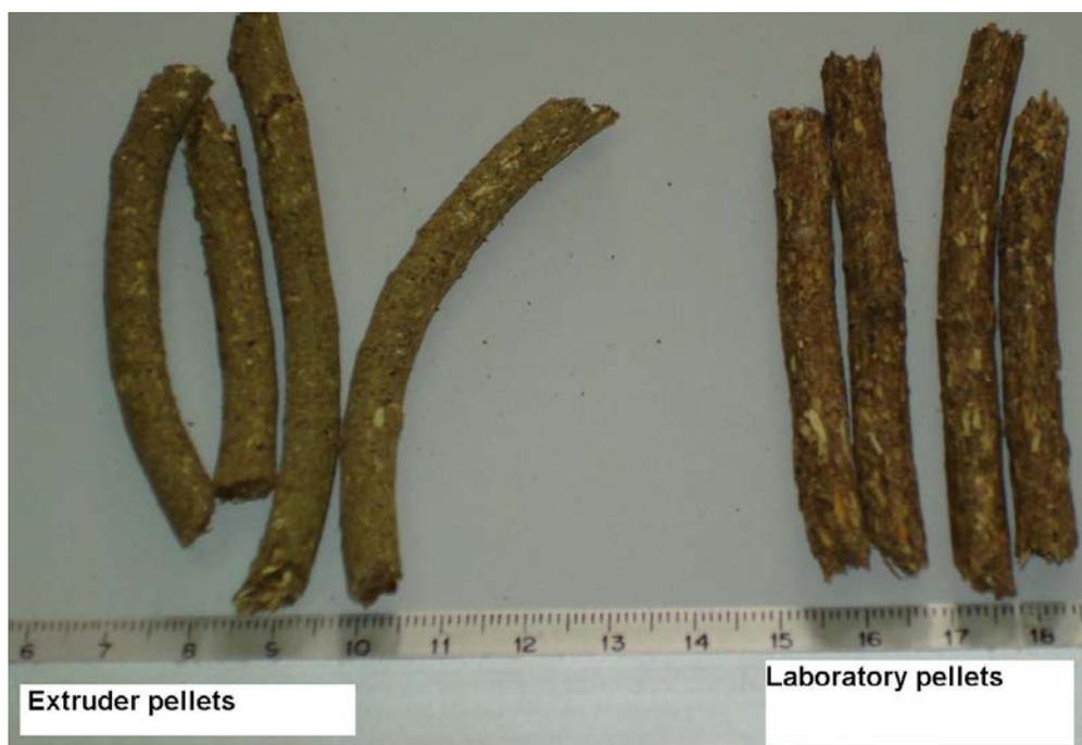
Figure 6. Comparison of pellets from the full scale extruder and from the laboratory.
