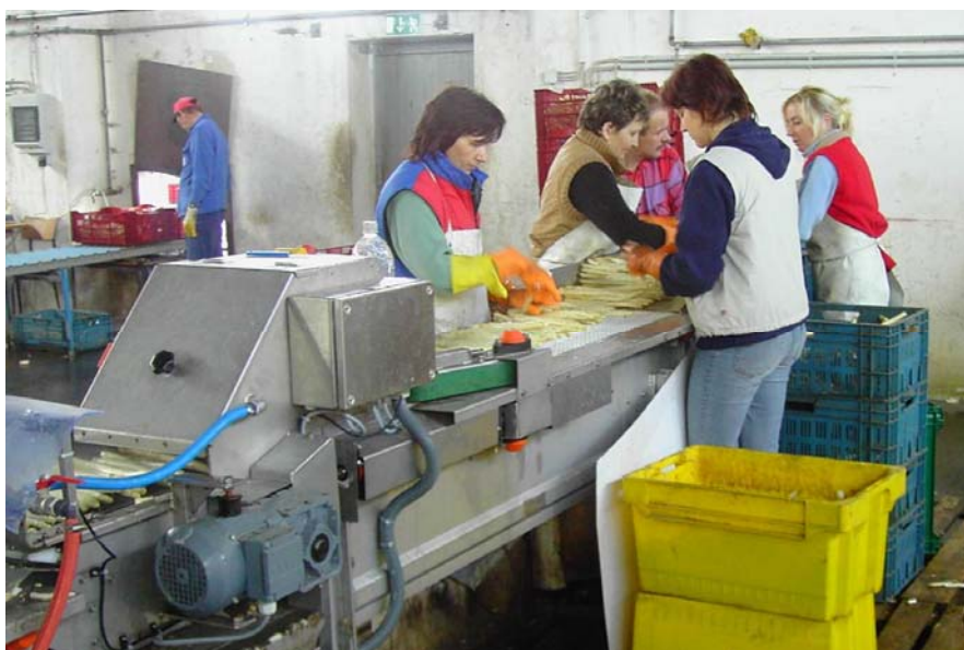
Figure 1. Manual supply of white asparagus for automatic washing and sorting
