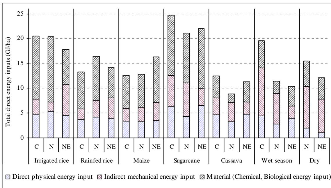
Figure 4. Total energy input for different crops in each region (C=the Central plain, N=the North and NE=the Northeast)
