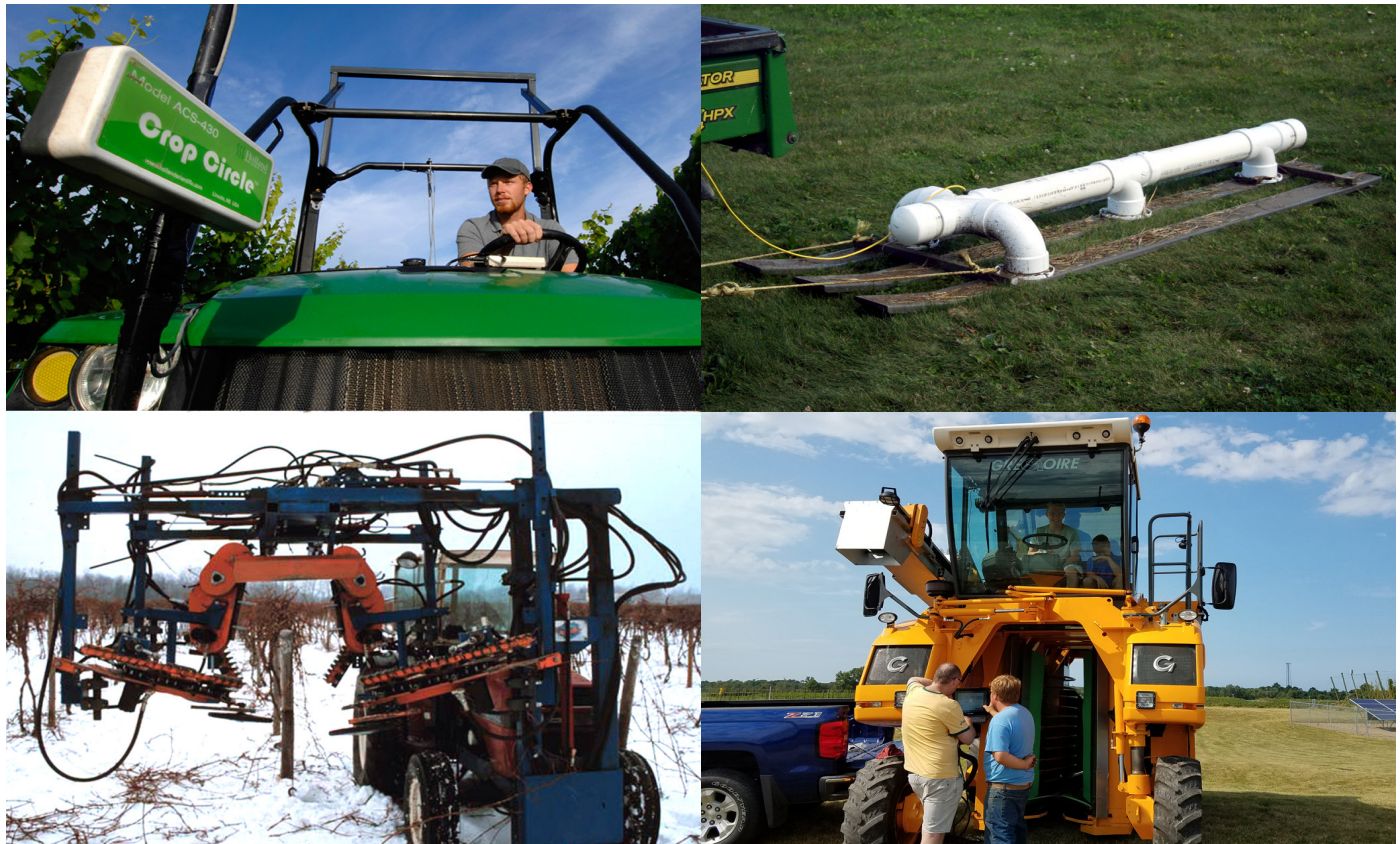
Figure 1. Equipment used for sensing and variable-rate crop thinning (clockwise from bottom left): Modified Morris-Oldridge mechanical pruning machine, Crop Circle NDVI sensor, DualEM soil sensor, and Gregoire mechanical harvester.
