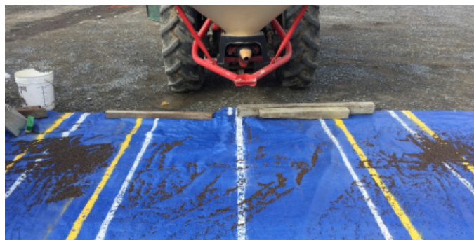
Figure 6. Vicon spreader with banding spout and simulated vineyard row. Parallel white lines on either side of the center line represent the area under the trellis with 8' row spacing. Yellow lines represent 9' row spacing. Photo by Hans Walter-Peterson
