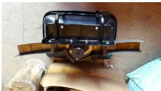
Figure 7. Underside of rotary spreader showing shroud around the rotor and side discharge chutes. Photo by Hans Walter-Peterson
