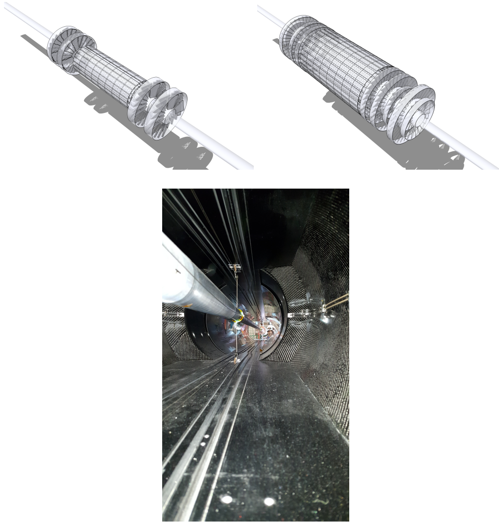
Figure 3.10: CAD schematic of the previous phase-0 pixel detector (top left), the upgrade phase-1 pixel detector (top right), and a photo of the volume in which they occupy within the CMS detector (bottom).
