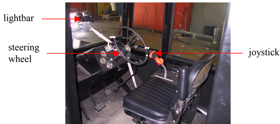
Figure 2. Interior view of the operator's station of the simulator showing the locations of the lightbar, steering wheel, and joystick in relation to the seat.
