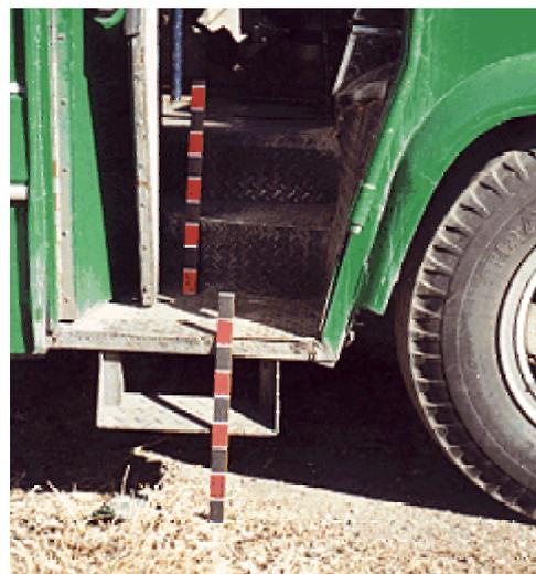
**Photo 5 Extra step installed under front door of *micro*, Mexico City**
