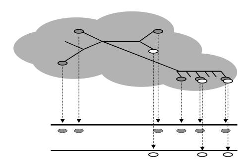
Figure 2: Two virtual networks overlayed upon one physical one. The overlay hides the structure of the physical network and may offer guarantees, such as isolation from interference or minimum bandwidth. The network shown would be incapable of offering fault-tolerance to router or link failures, because the underlying physical infrastructure lacks redundancy.
