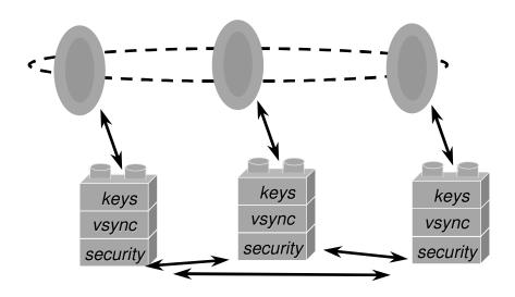
Figure 3: At each of the endpoints of a group (a VON), a stack of protocol elements assists in transforming the properties of the underlying ON into the desired VON properties. The application process would not normally be directly aware of the behavior of the protocol stack. The stack shown supports a model called "secured virtual synchrony" over which security keys might be managed on behalf of the application. VONs with different roles and properties might use different stacks.
