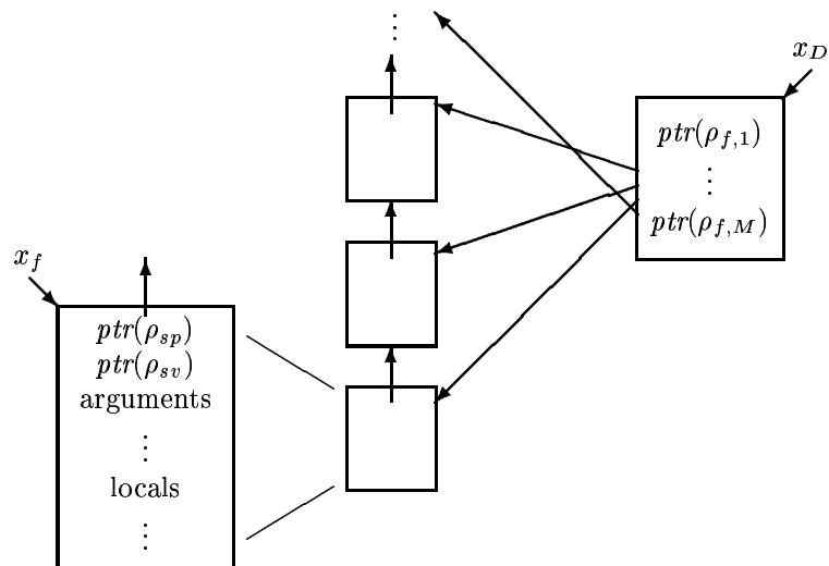
Figure 7: Snapshot of the stack and display during the execution of a translated program.
