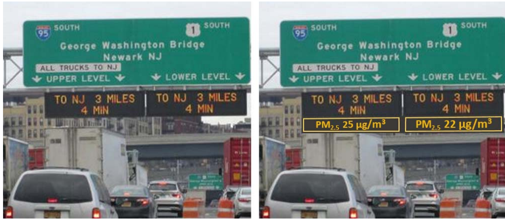
Figure 2.1: DMS at the George Washington Bridge (GWB). Travel time information (left panel), source: http://www.panynj.gov . The information of average PM_{2.5} concentration on each level of the GWB are “added” artificially (right panel).
