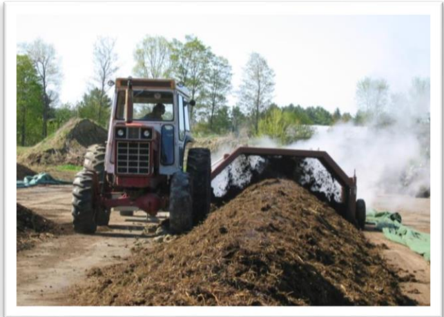
Tractor-pulled compost turner (photo by Mark King)
